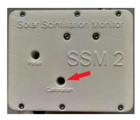
Turn the screw on the trimmer resistor with a small slotted screwdriver so that the input signal is approx. 1 Volt to 1.15 Volt. Caution During this calibration, the sensor must point directly into the sun (no clouds).
